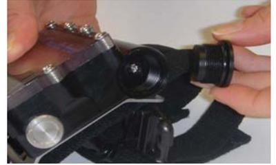
Carefully pull out the battery holder. To prevent battery bounce and rattling, it's fitted tightly, so you will need something like a dental pick or a paper clip to pull out the holder.
