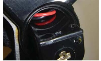
Inspect and, if necessary, apply a light coat of silicone to the O ring in the battery cap. Reinstall the battery cap taking care not to pinch or deform the O ring.
