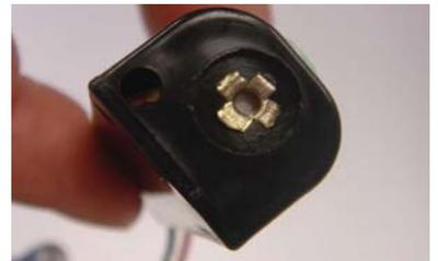
The bottom needs to be aligned with the wires as they feed through the case. Carefully fold the wires along the bottom of the holder and insert back into the compartment. Care must be taken not to pinch and score the wires.
