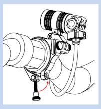
Also, the same two-hole screw mounting configuration as the NERD 1 is retained (e.g. rEvo and JJ mounts).
