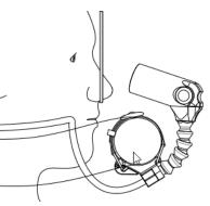
Alternate mounting was possible using two screw holes (e.g. rEvo and JJ mounts).
