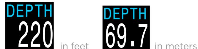
In feet, depth displays with no decimal places. In meters, depth displays with one decimal place up to 99.9m.
