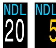
The time remaining, in minutes, at the current depth until decompression stops will be necessary. Displays in **Yellow** when the NDL is less than the low NDL limit (Default 5 minutes).
