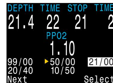
New style gas select menu layout. 5 gases currently programmed and on
