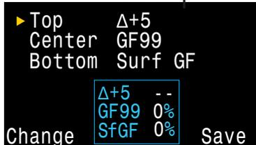
The Perdix 2 has a mini display function that allows it to show 3 pieces of information in each of the left and right custom slots at the expense of font size.
