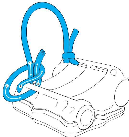
When using bungee or shock cord, always create two independent loops so that a single break will not result in a lost dive computer.
