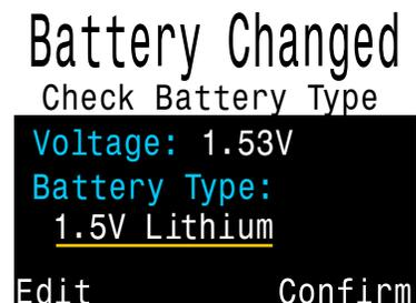
The Perdix 2 can accept most AA sized (14500 size) batteries that output a voltage between 0.9V and 4.3V. However, some batteries are better than others.
