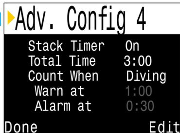
It can be toggled on and off in the Advanced Config. 3 menu. The total time can be set anywhere between and 1h and 9h 59m. The stack timer can be set to count down either when diving, or when the computer is ON. A warning will alert the diver when the stack timer has 1h remaining and an alarm will be displayed when the stack timer has 30 minutes remaining.
