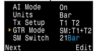
GTR and SAC are only based on one tank, or on two tanks in sidemount configuration. Note that for sidemount the tanks must be of identical volume for SAC to be accurate.
