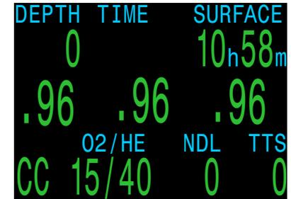
This is because weather causes minor changes in barometric pressure. For example, say a low-pressure weather system has reduced the normal (1013mbar) barometric pressure to 990mbar. The PPO2 in absolute atmospheres is then  $0.98 * (990/1013) = 0.96$ .
