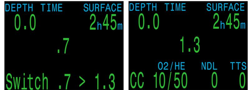
For closed circuit diving the Petrel 3 operates in internal PPO2 mode. This mode is used to calculate decompression for an unconnected rebreather.
