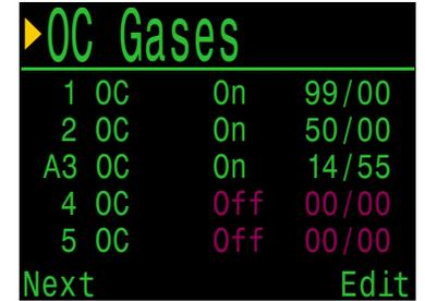
Each gas can be turned on or off and set to any concentration of O2 and helium. The remaining percentage is assumed to be nitrogen.
