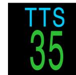
The time-to-surface in minutes. This is the current time to ascend to the surface including the ascent plus all required deco stops.
