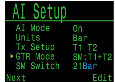
GTR and SAC are only based on one tank, or on two tanks in sidemount configuration. Note that for sidemount the tanks must be of identical volume for SAC to be accurate.
