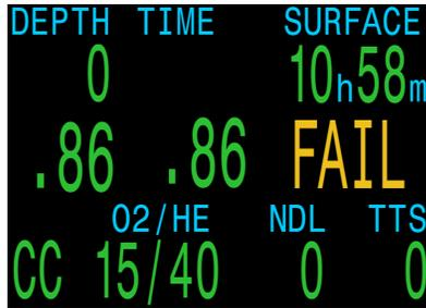
**All sensors display FAIL after calibration**
