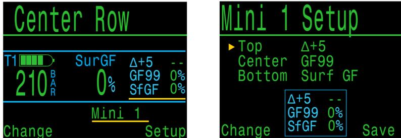
The Petrel 3 has a mini display function that allows it to show 3 pieces of information in each of the left and right custom slots at the expense of font size.
