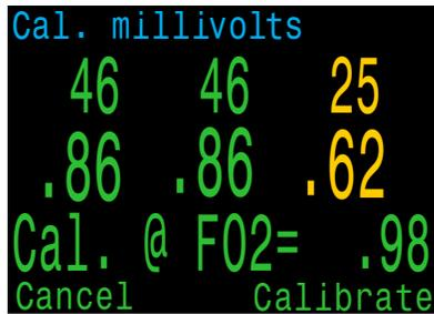
If you need to change the calibration gas FO<sub>2</sub>, do this in the System Setup O<sub>2</sub> Setup menu.
