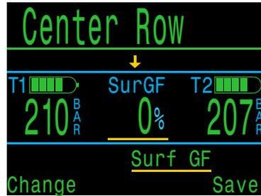
When using internal setpoint, only the left and right positions are configurable in CC/BO mode as the middle position is reserved for PPO2 Setpoint.
