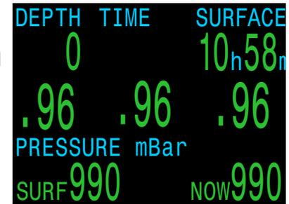
The 0.96 PPO2 result is, in this case, correct. At high altitudes, the difference between FO2 and PPO2 will be even larger. To see the current pressure, start at the main screen and press the SELECT button a few times (displays as Pressure mBar NOW).
