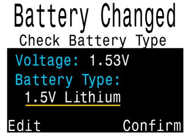
The Petrel 3 can accept most AA sized (14500 size) batteries that output a voltage between 0.9V and 4.3V. However, some batteries are better than others.
